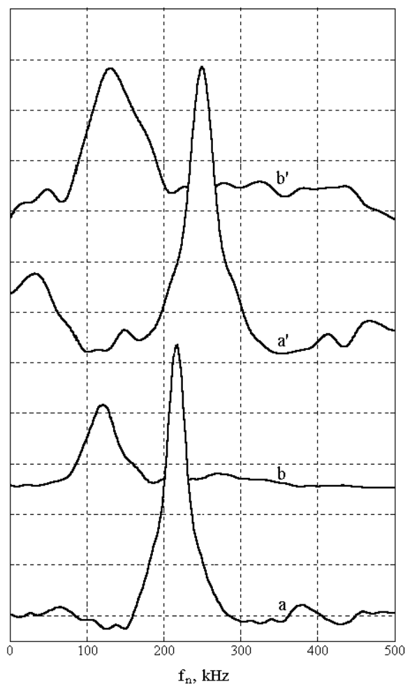
Fig. 13. 1D-nutation spectrum in the coordinates a) f_{n1} and b) f_{n2} .
